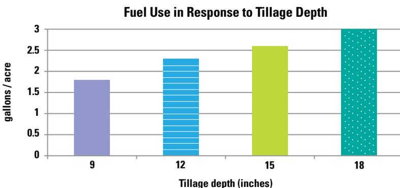
Figure 3. Diesel fuel used at different depths for subsoiler operation (Shinners, 1989).
