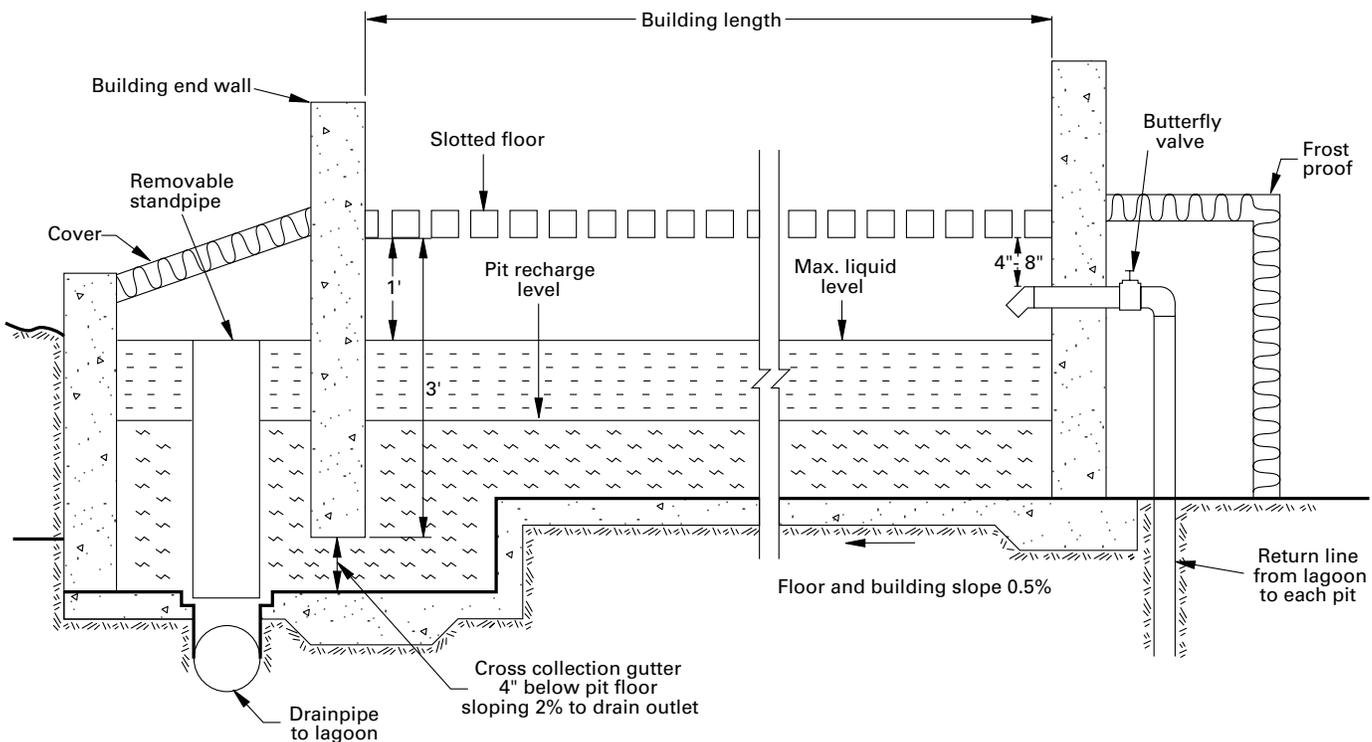
**Figure 2. Cross-section of a pit recharge system**
