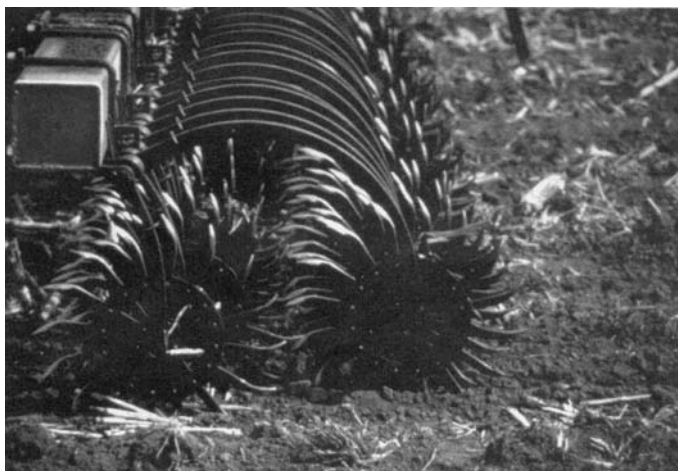
A 20-inch spacing between hoe gangs helps handle residue. The rear gang cleans the front one.
