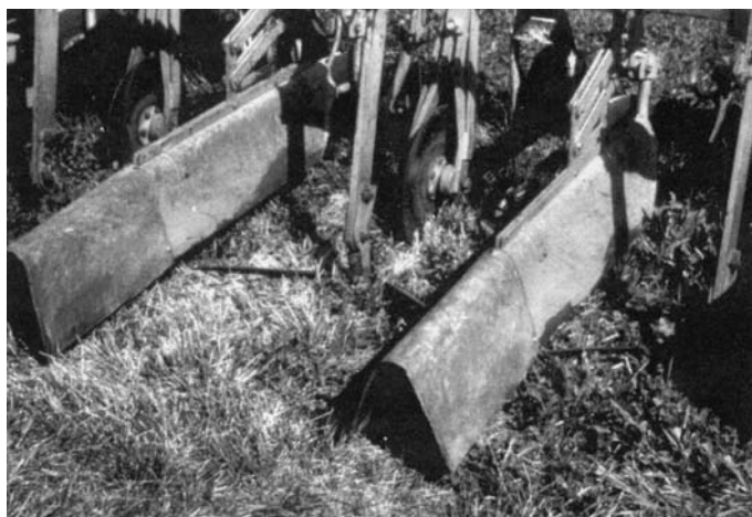
Extension on tent shields drag the ground to protect the young crop at first cultivation.
