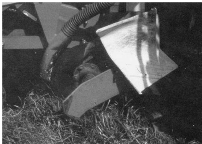
Side plates clean ridge shoulders. Plastic covers prevent weed seeds from falling back into row. Alternatively, extensions can be welded to planter sweeps to help bury weeds, manure, and cover crops between rows.
