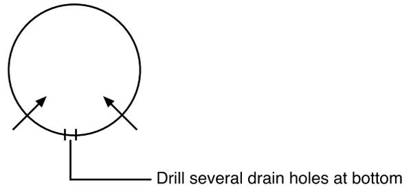
**Figure 1. Drill holes in lower quarter of tube.**
