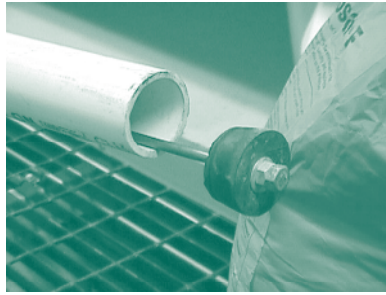
Figure 3. Rubber stopper attached to a metal rod to serve as a stopper for PVC manure sampling tube.
